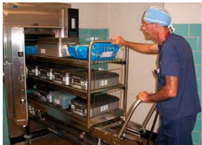
A sterile processing technician pushing a cart of unsterile instruments into a steam sterilizer
