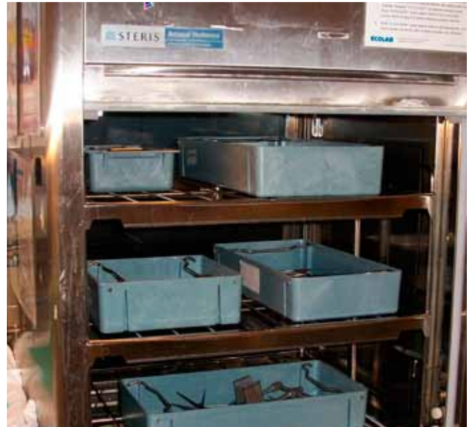
A washer-disinfector is loaded with dirty surgical instruments. Once the door is closed and a cycle is selected, the instruments will be mechanically decontaminated
