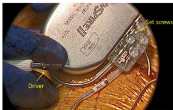
Fig. 3 Implantable pulse generator (IPG) has two 3.2 mm low profile connector ports (STIM port, SENSE port) which house the stimulation and pleural pressure sensing lead connectors. The lead connectors are secured with set screws using a driver
